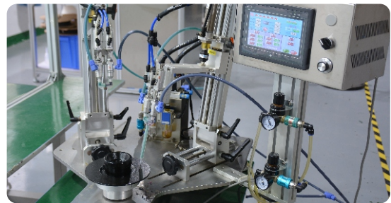
LF Automatic Production: Computer-controlled Dispensing Machine
