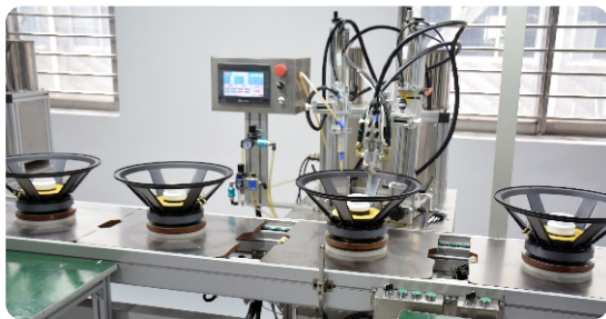
LF Automatic Production: Computer-controlled Dispensing Machine
