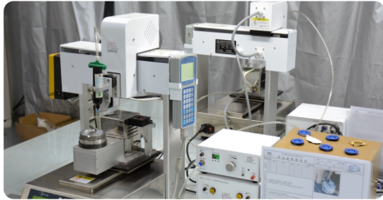
Compression Driver Production: Dispensing with four-axis Robot
